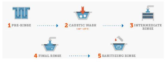
Fig. 3.3.1: Flow Diagram of CIP cycle
